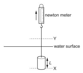
The cylinder, of height *L*, is slowly raised vertically by lifting the newton meter.
